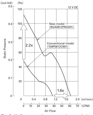
Fig. 5: Air flow vs static pressure characteristics between our conventional model and the new model
