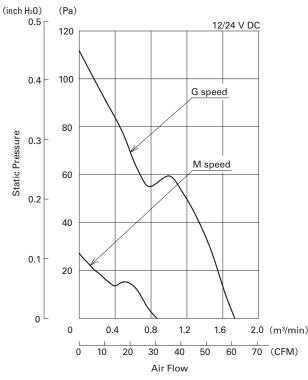
Fig. 3: Air flow vs static pressure characteristics
