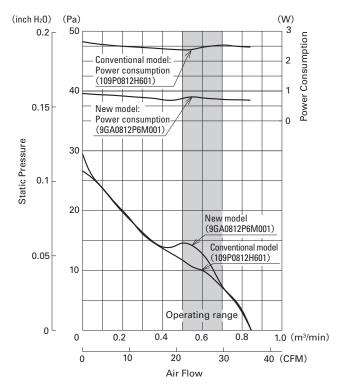
Fig. 6: Comparison of air flow vs static pressure vs power characteristics
