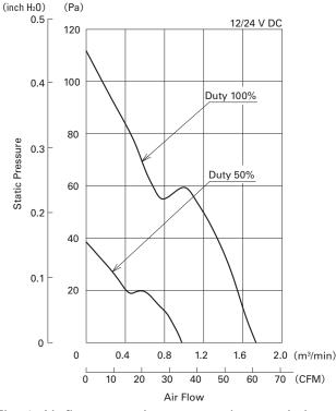
Fig. 4: Air flow vs static pressure characteristics at individual PWM duty cycle
