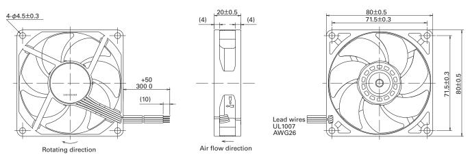
Fig. 2: "San Ace 80" GA type dimensions (unit: mm)
