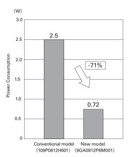
Fig. 7: Comparison of power consumption at free air
