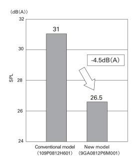
Fig. 8: Comparison of SPL during free air conditions
